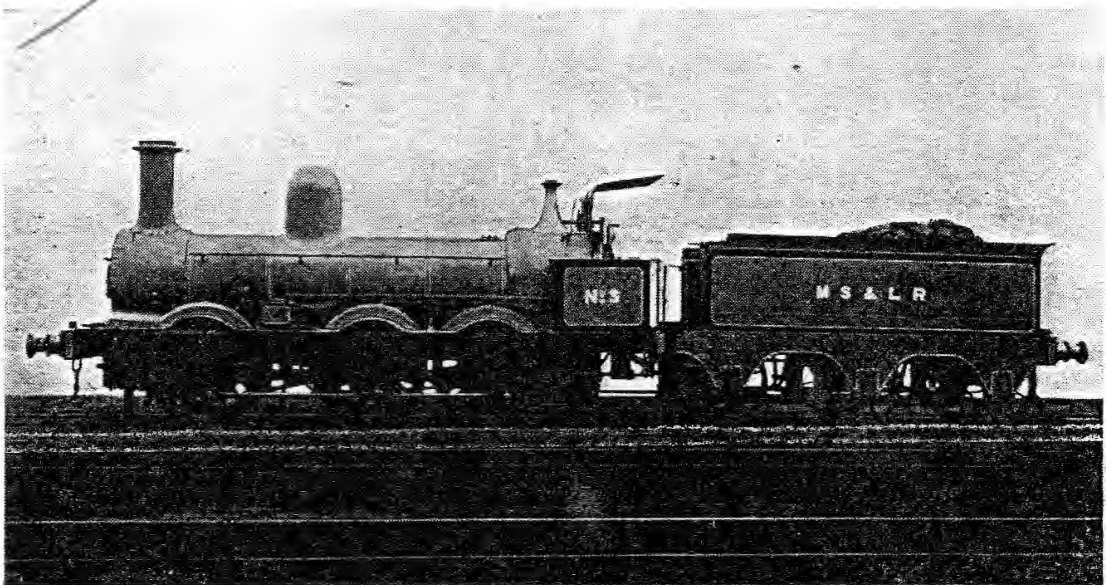
M.S. & L. 0-6-0 No. 3 (originally built for S. A. & M. in 1847) as rebuilt 1864.
